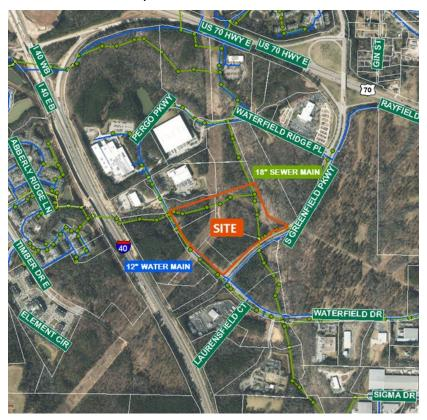
**Stormwater Management:** Greenfield 27 is a commercial development that is not located within the watershed protection area. This site is subject to water quality requirements for nitrogen and water quantity requirements for the 1, 10 and 25 year storm events.
