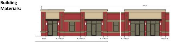
POL JOINT NOTE: "MCJ" INDICATES MASONRY CONTROL JOINTS ADJACENT PILASTERS (TYPICAL/U.N.O.)
