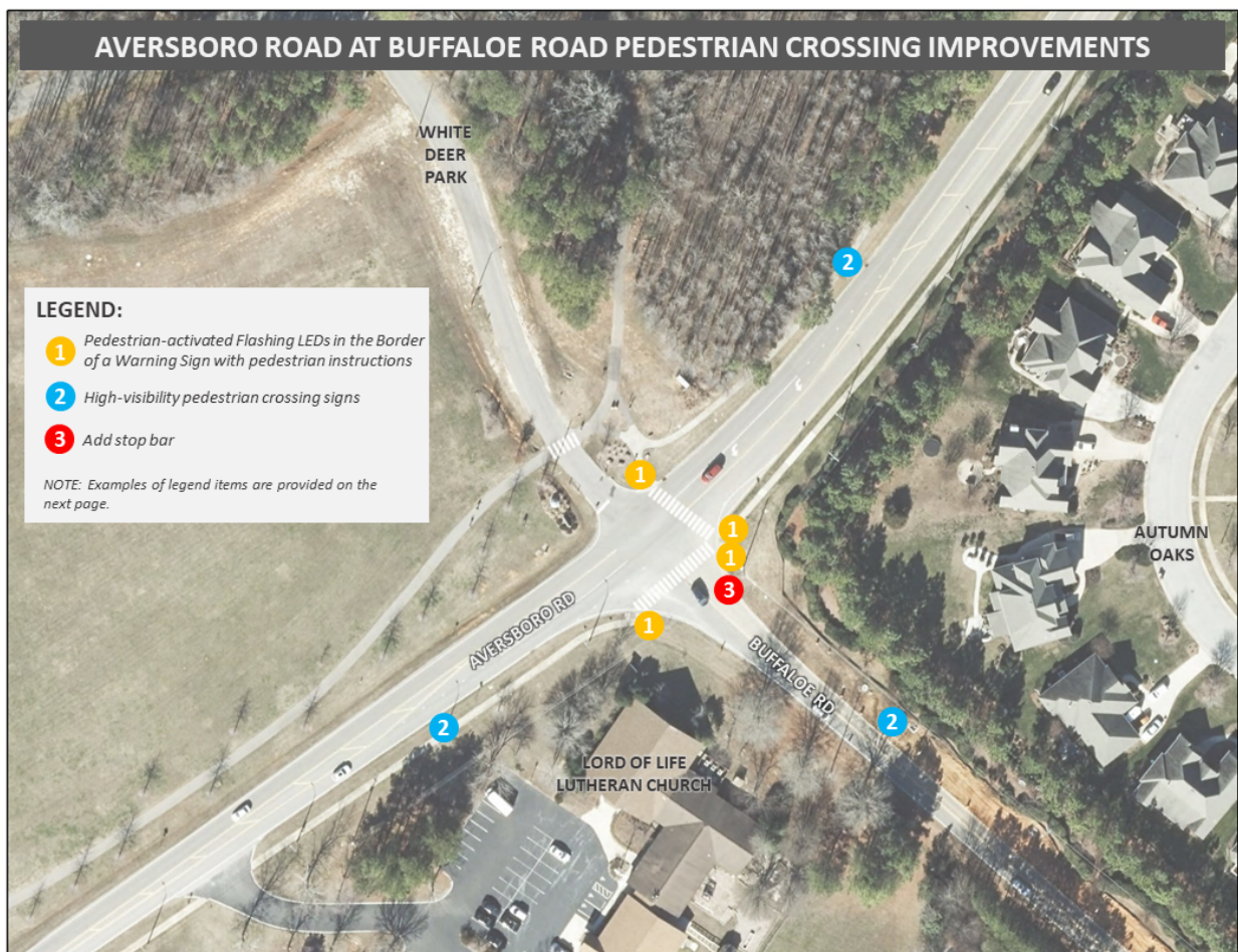
Figure 1: Aversboro Road at Buffalo Road Potential Pedestrian Crossing Improvements
